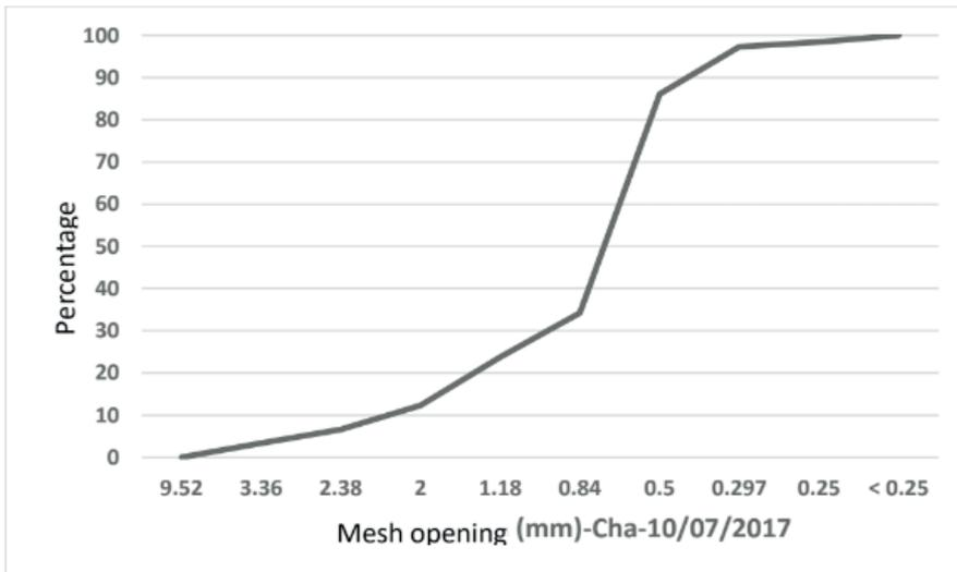
Figure 1.- Typical granulometric curve
