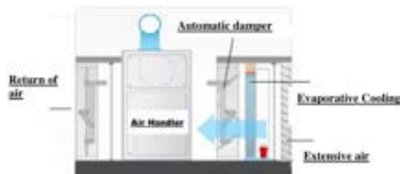
Figure 3 - Example of the evaporative system diagram (external air temperature between 16°C and 25°C or enthalpy below 12.5 kcal/kg)
