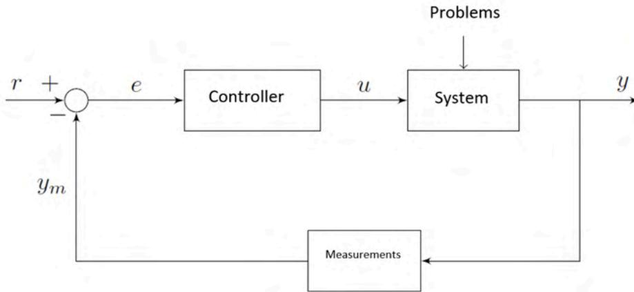
Figure 1: Control loop:PID
