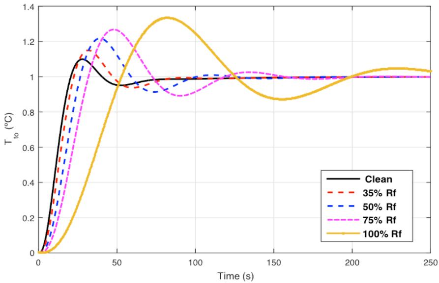
Figure 3: Response to step disturbance before setting controller parameters
