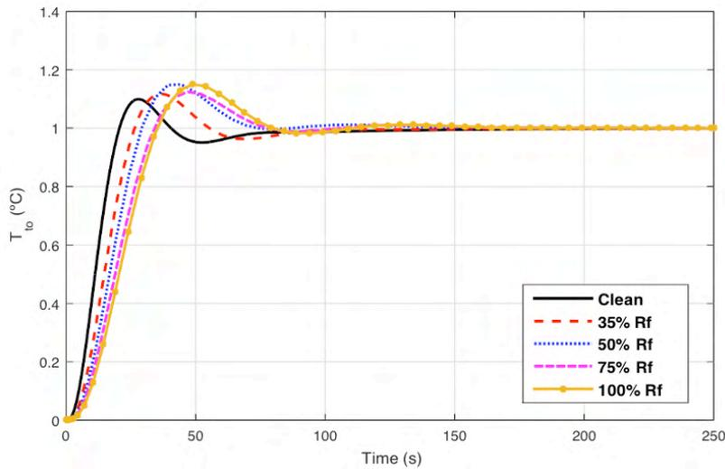
Figure 4: Response to step disturbance after adjusting controller parameters
