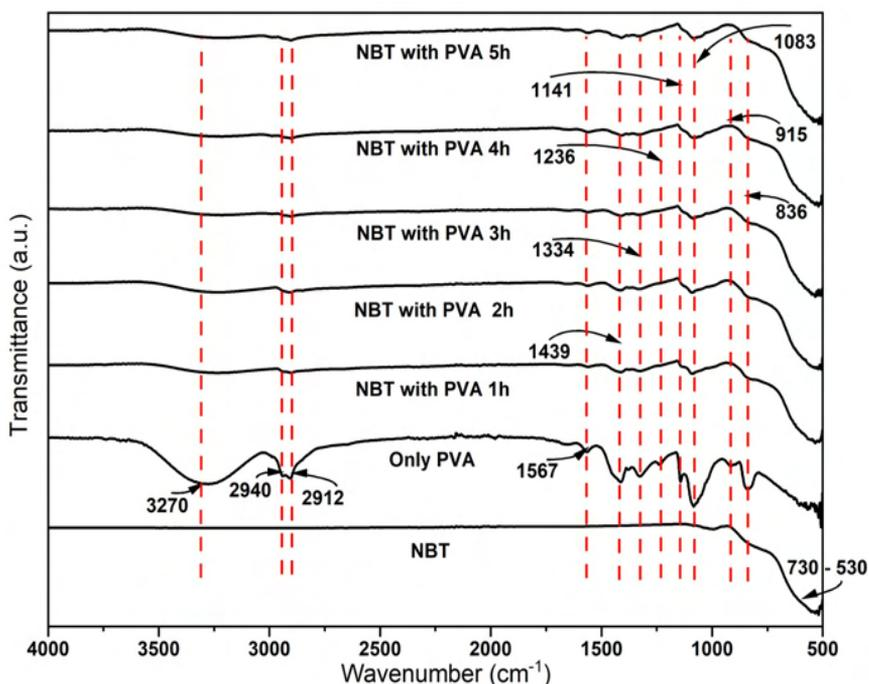
Figure 4. - FTIR spectra of the NBT ceramic system under different milling times incorporating PVA.
