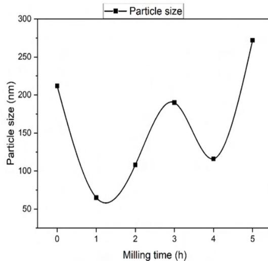
Figure 3. - Particle size populations of ceramic powders under different milling times incorporating PVA.
