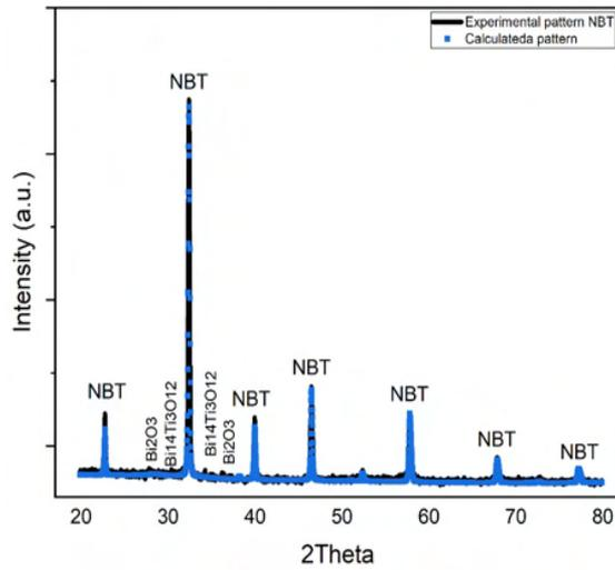
Figure 1.- Diffraction pattern of the NBT ceramic system.
