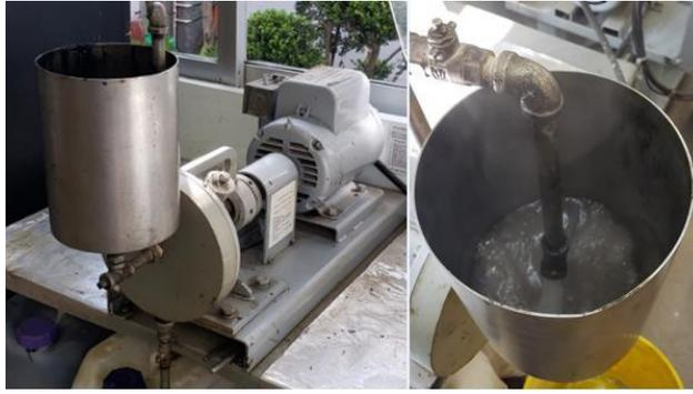
Fig. 1 Colloid mill used to reduce asphalt particle size and emulsify it.
