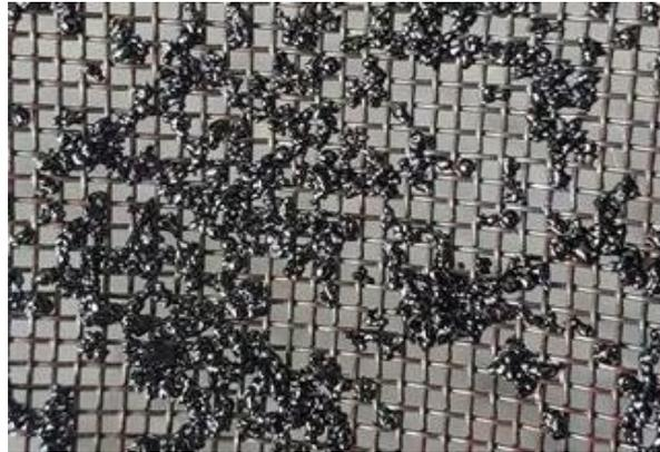
Fig. 4. Mesh of test of sieve residue of the sample 40-3.
