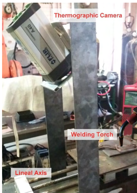
Figure 3: Flat welding table and instruments support
