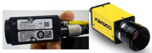
Figure 5. Camera model used: Cognex, In-Sight micro 1400 model.
