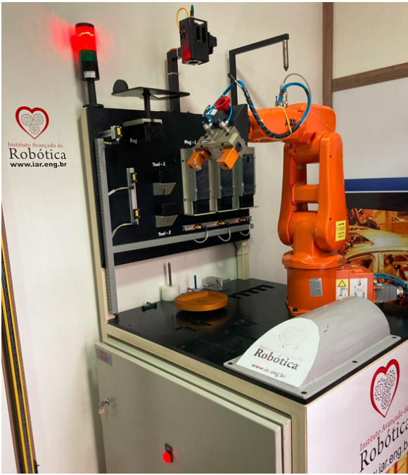
Figure 9. ABB Robotic Cell.
