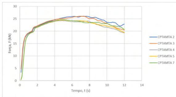
Figure 11 - Pressing Force x Time CPTAMTA Chart
