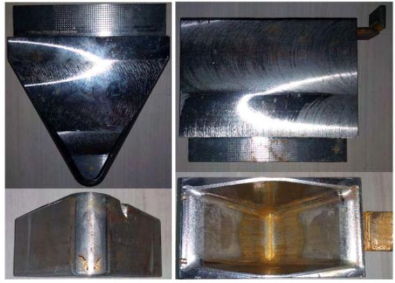
Figure 6 - Machined Upper and Lower Die.
