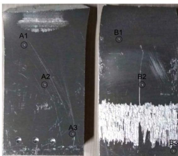
Figure 15 - Hardness Measurement Points/
