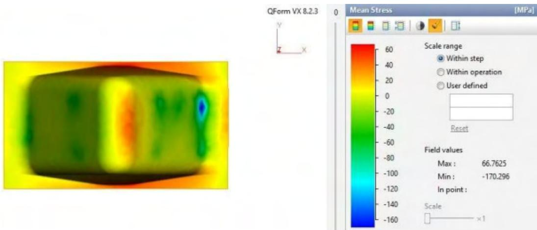
Figure 4 - Main Stresses in the Lower Matrix.
