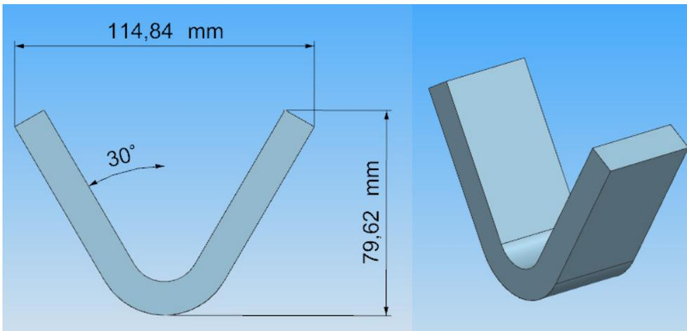
Figure 3 - Specimen After Deformation.
