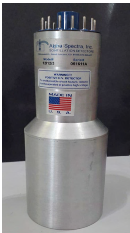
Fig. 5 - High precision Gamma Detector. Sodium Iodide crystal [NaI(Tl)]doped with Thallium.
