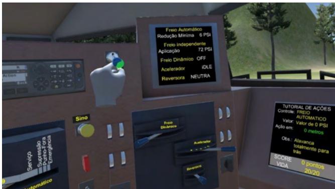
Figure 2. Use of the Oculus Touch to manipulate the horn lever in the locomotive panel.
