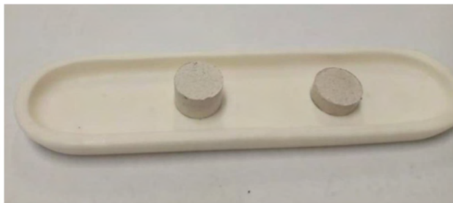
Figure 13 – Formed powder pellets before being taken to the electric oven to obtain the glass.
