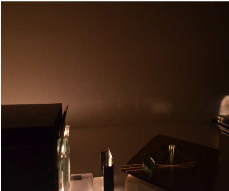
Figure 15: Multiple reflections of light passing through ellipse its foci.
