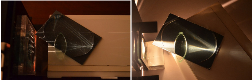
Figure 16: Ellipse projecting parallels beams.
