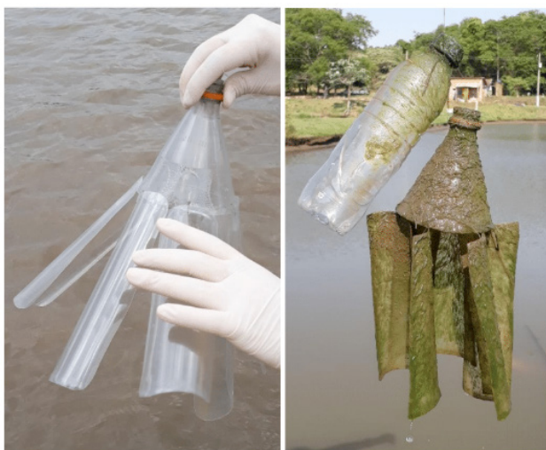
Fig. 2: Prepared PET strips before and after 30 days submerged at the fish farming collection points.
