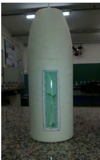
Figure 2: Expandable polystyrene container (Styrofoam) with the beaker and thermometer, and the PET bottle. The beaker was used to mix the acid with the base.
