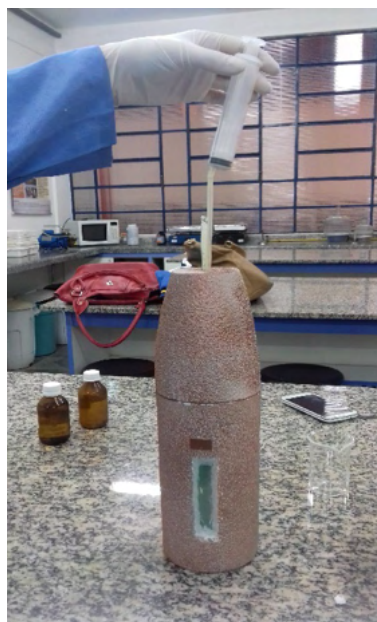
Figure 4: Point-to-use calorimeter, with all the necessary materials attached to the expandable polystyrene container.
