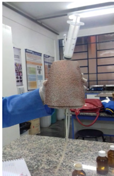
Figure 3: Attaching the syringe and thermometer to the calorimeter cover.
