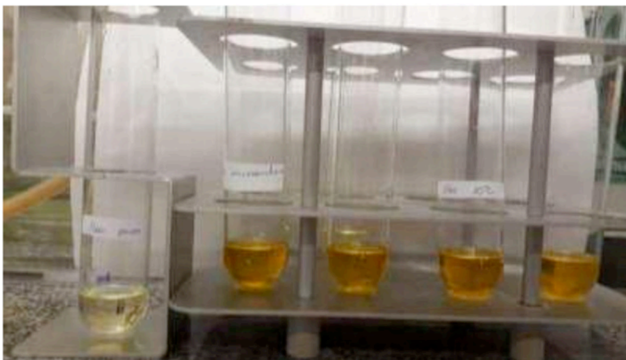
Figure 2 - Color difference between in natura soybean oil and oil incubated at 10 °C with dried flowers in microwaves
