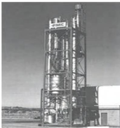
Figura 13. Evaporador TASTE (*Thermally Accelerated Short Time Evaporator*).
