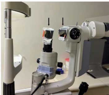
Figure 1: Slit lamp prototype with two polarized filters (black arrows), orthogonal to each other.
