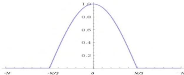
Fig. 5: Normalized cosine exponent of the exponential function in von Mises window: the (entire) cosine \cos(\pi t/N) is periodic in [-N, N] , but the support is confined within [-N/2, N/2] due to the rectangular pulse.
