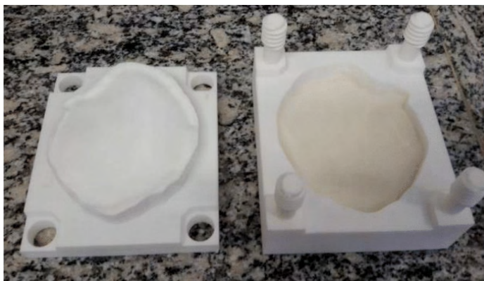
Figure 5. Bone cement applied to the prostheses mold.
