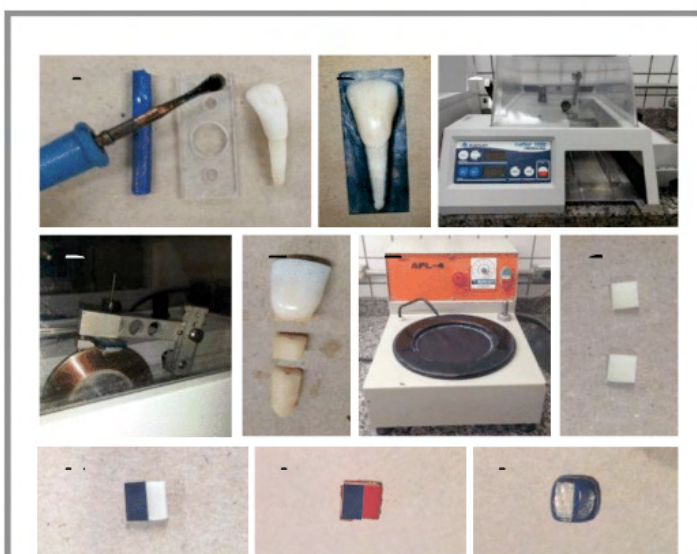
Figure 2. Preparation of specimens. A) Materials used to fix the tooth on the acrylic plate. B) Tooth fixed with sculpture wax. C) Cutting Machine - ISOMET® 1000. D) Tooth being sectioned. E) Sectioned fragments. F) APL-4 polishing machine. G) Standardized specimens. H) Isolation of half of the specimen's surface. I) Specimen after application of two layers of red cosmetic enamel. J) Specimen ready to receive treatment.
