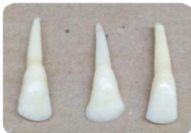
Figure 1. Selection of bovine incisors. Cleaned with periodontal curette; immersed for 7 days in 10% formalin; stored in distilled water at 4 ° C.
