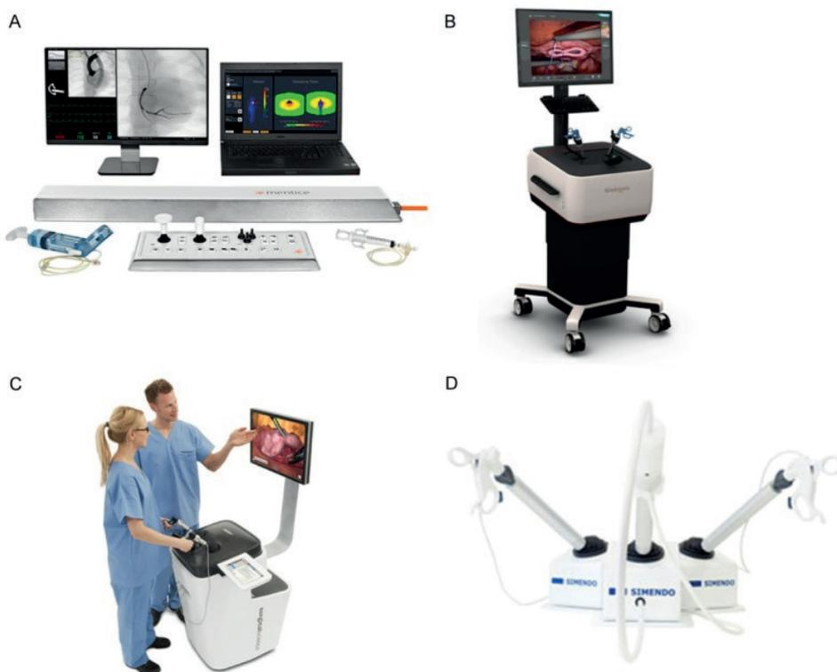
Figura 1 - Simuladores: MIST-VR (A), Lap Mentor (B), Lap Sim (C) e Simendo (D).
