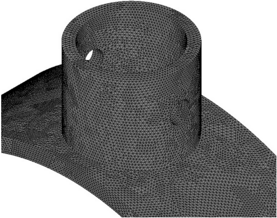
Figure 6. Mesh for the transition cylinder-legs of the fork. Source: own authorship (2020).
