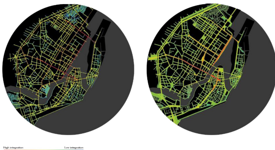
Figures 4 and 5. Global integration of the city center of Recife - axial map and all lines axial map (from left to right).
