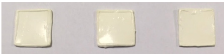
Figure 4. Test Specimens, Carbon steel AISI 1010 painted with epoxy coating.
