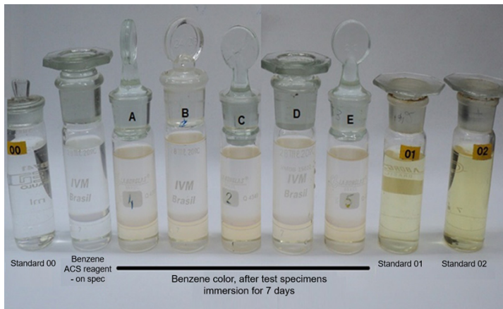
Figure 7. Samples of benzene ACS reagent and benzene after TS immersion (A to E), painted with Formulation 2.
