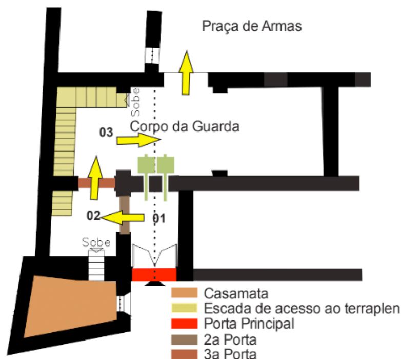
Figure6-Circulation scheme through the gateway.
