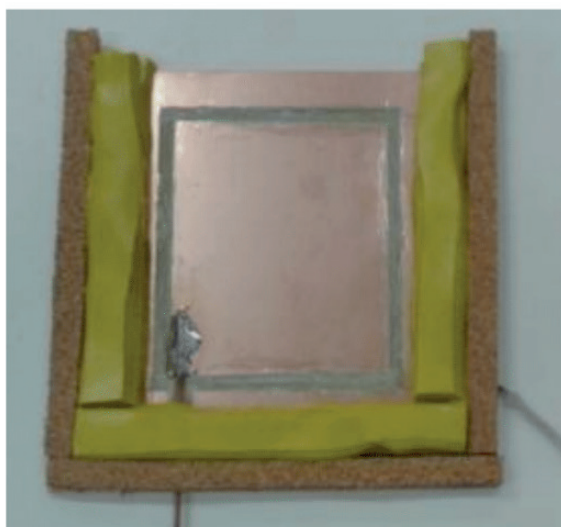
Figure 2. Tacky tape was used as sealant and cork as spacer
