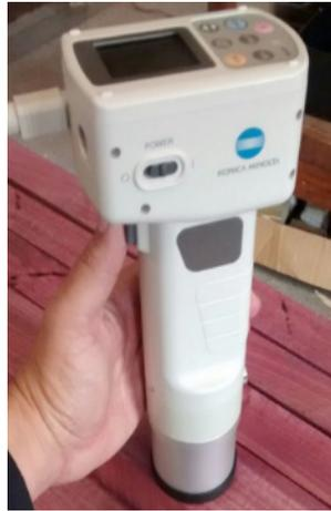
Figure 1 – Konica Minolta portable colorimeter.
