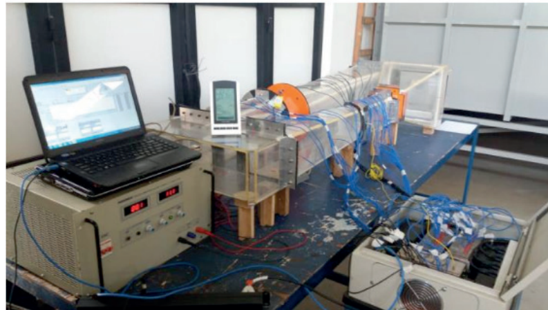
Figure 15 - The wind tunnel built for the project. By the authors.
