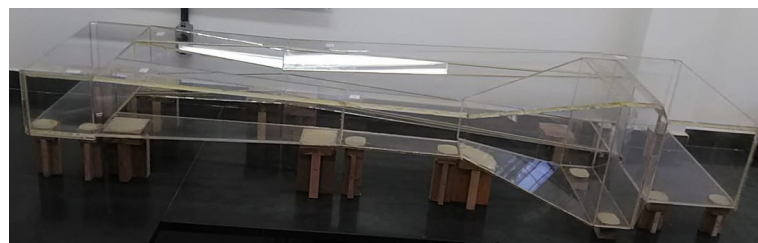
Figure 10 - The acrylic pieces glued with epoxy. By the authors.
