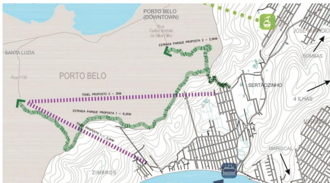
Figure 2 - Alternatives to new access of Bombinhas. In Green, the road over Zimbros Hill and, in purple, the two path option for a tunnel.
