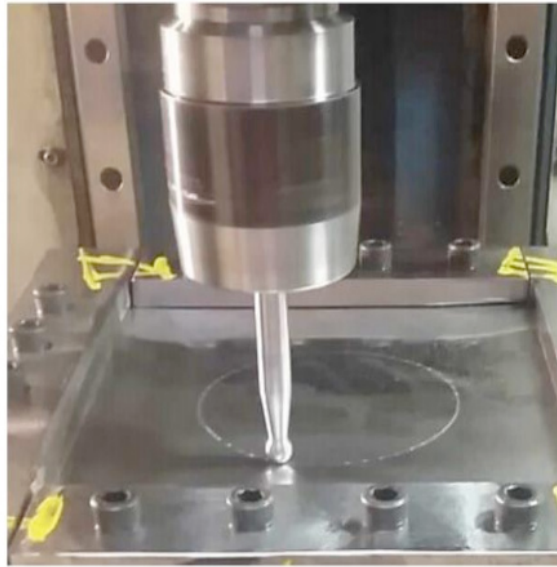
Figure 2. Hemispherical tip tool fixed at the mandrel at CNC machine.
