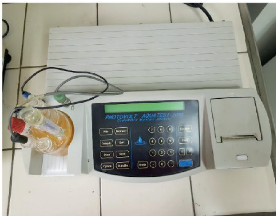
Image 3. Photovolt Aquatest 2010, Karl Fisher method. Source: Parker Hannifin
