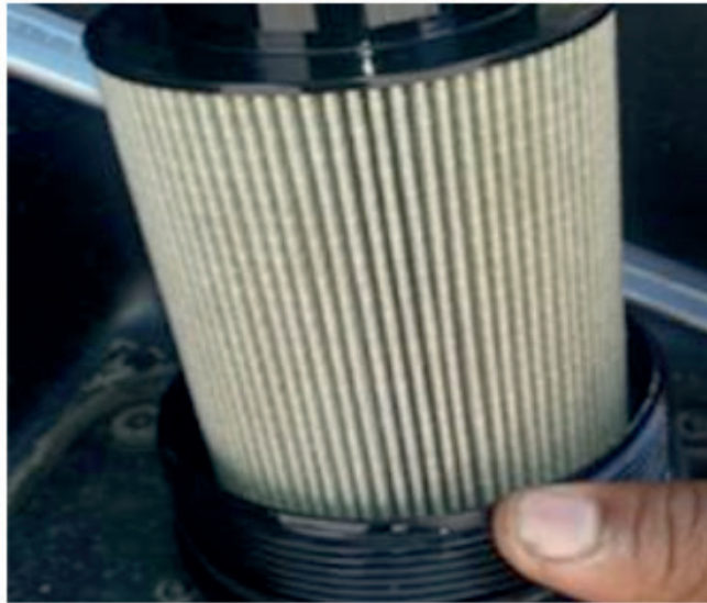
Image 4. Filtering element media after test with diesel S 10 B10 with 46 hours of oxidation stability. Water separation efficiency with 90% in average. Source: Volkswagen Truck & Bus.
