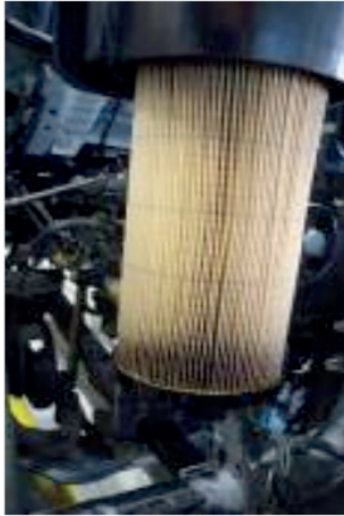
Image 6. Filtering element media after test with diesel S10 B15 with 4,5 hours of oxidation stability. Water separation efficiency with 34%. Source: Volkswagen Truck & Bus.
