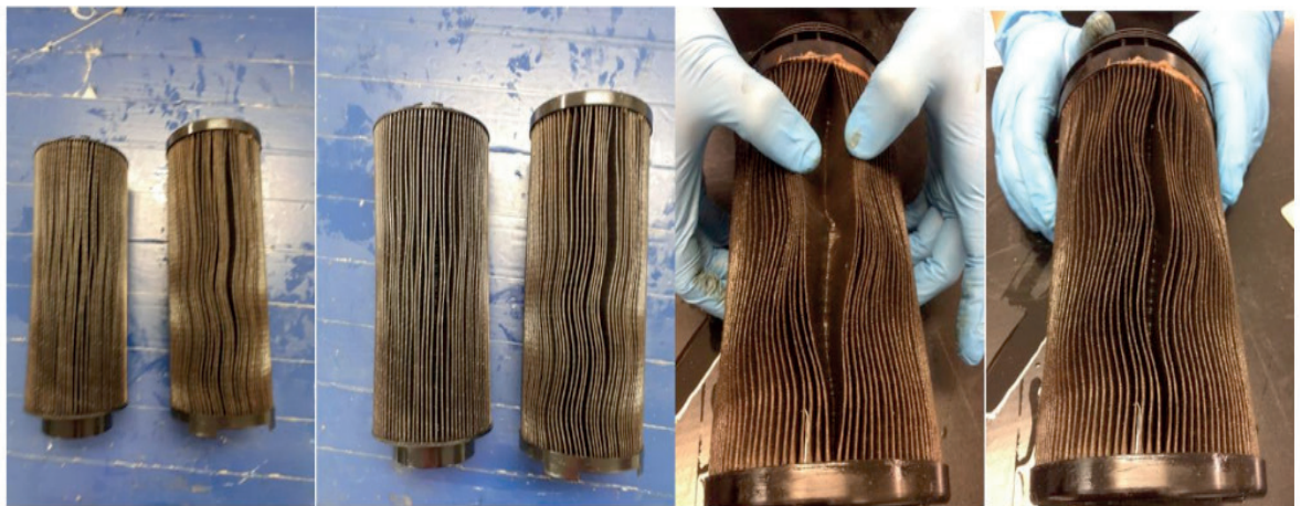
Image 5. Filtering element media after test with diesel S 500 B10 with 14 hours of oxidation stability. Water separation efficiency with 50% in average. Source: Volkswagen Truck & Bus.
