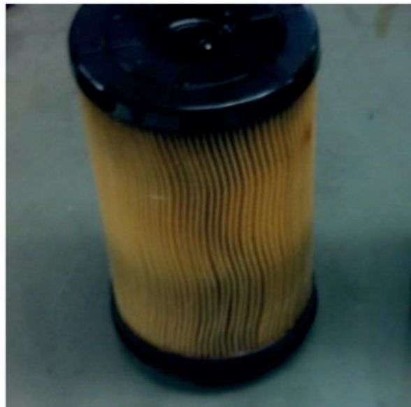
Image 7. Filtering element media after test with diesel S10 B15 with 27 hours of oxidation stability. Water separation efficiency with 95,5%. Source: Volkswagen Truck & Bus.
