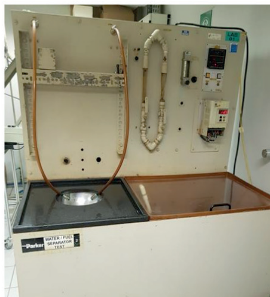
Image 2. Water separation test bench analysis according to SAE J1839. Source: Parker Hannifin
