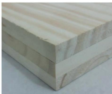
Figura 1: Amostra de CLT.
