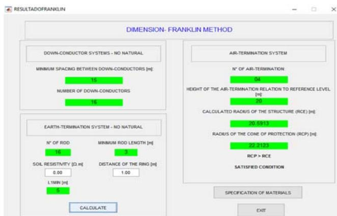
Fig.10: Result of the simulation by the Franklin method.
