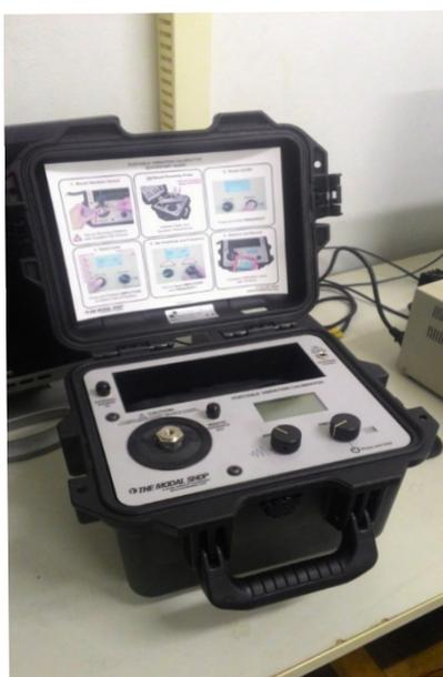
Figura 5. *9100D Portable Shaker Vibration Calibrator*.
