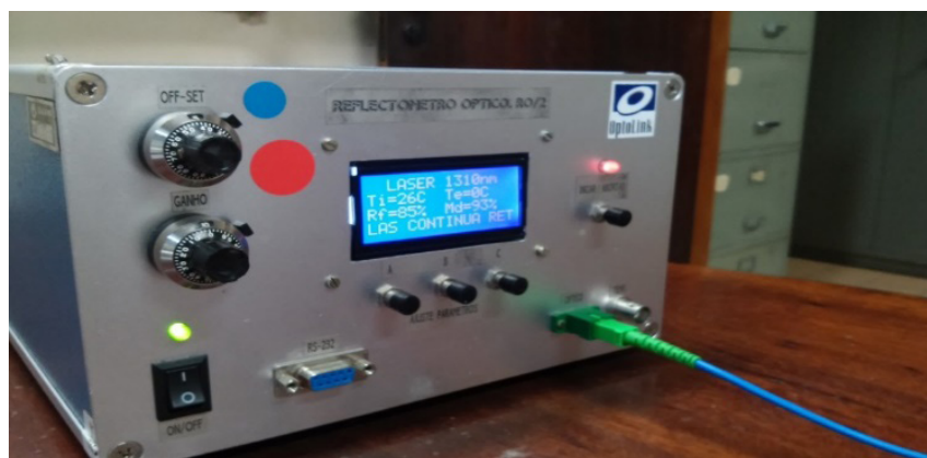
Figure 3. Optical fiber reflectometer used for analyses. The sensor unit consists of a 1310 nm laser launched through a single-mode waveguide. The signal that returns is directed by a coupler to a photodetector and is then processed and analyzed by computer routines.
