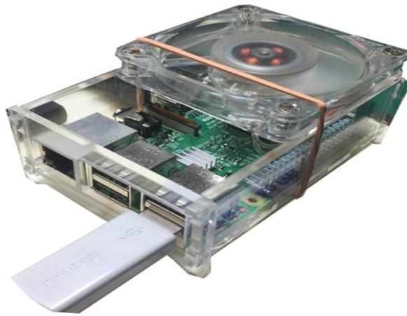
FIGURA 4: *Raspberry Pi 3* com cooler.
