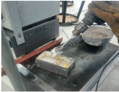
Figure 4. Photograph showing mechanical stirring during the production of the master alloys.
