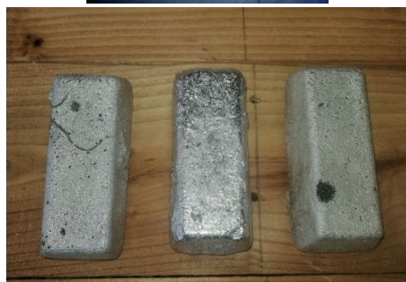
Figures 1 and 2. Photograph showing the melting of aluminum cans in a floor furnace and the production of ingots for the established study.
