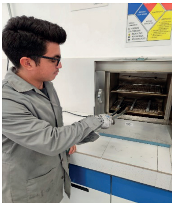
Figure 8. Aging and cooling to room temperature.
