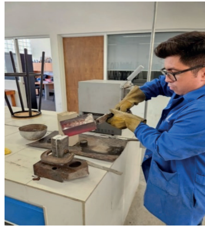
Figure 5. Modified with master alloy aluminum 6061T6 melting
