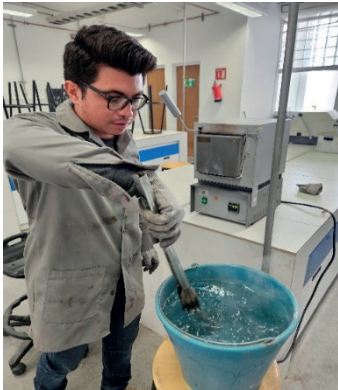
Figure 7. Solubilization and water quenching.
