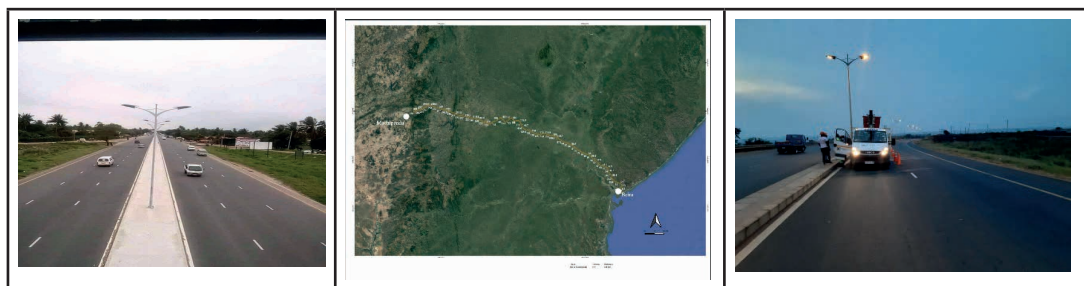
Figure 3. Route of the EN6, from Porto da Beira to the Machipanda border: two carriageways, three lanes in each direction, separated by a simple concrete central divider. Photos by the author, image from Google Earth.
