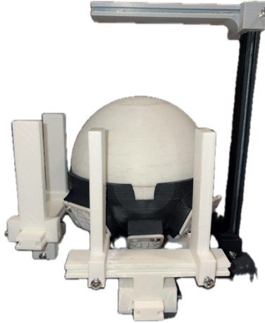
Fig. 8. Motion-tracking system 3D-printed structure.
