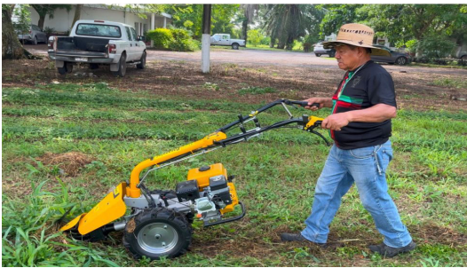
Figure 2. Speed test under field conditions with a Parazzini rototiller.
