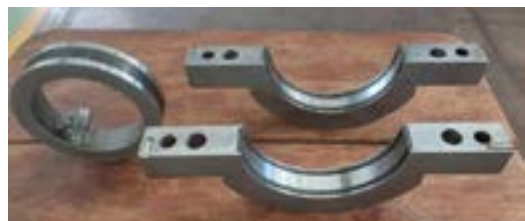
Fig. 5. (Prototype of the split container disassembled)Hydrostatic test of the split container prototype
