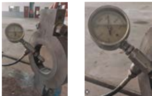
Fig. 6. (Hydrostatic test with 1.3x working pressure = 3,900 psi.)
